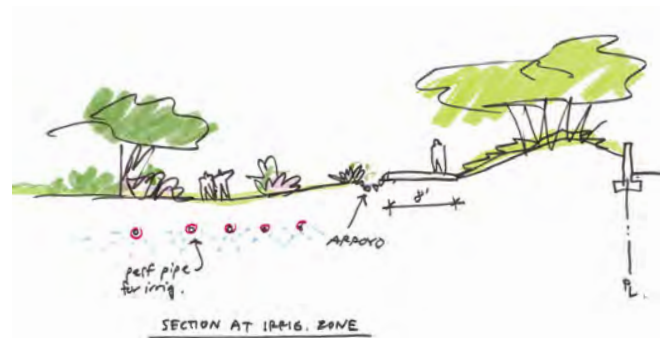
Perforated pipes deliver subsurface irrigation to the freshwater marsh/ meadow
